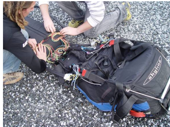
Pic. 70 pushing the lines into the d-bag
