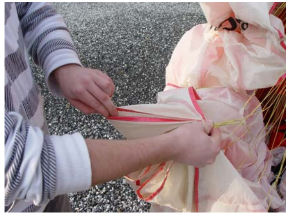
Pic. 17 the trailing edges should be pulled out neatly
