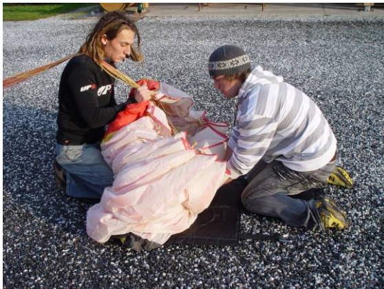
Pic. 35 Put the glider onto the d-bag
