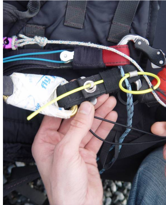
Pic. 63 and finally insert the releaser
