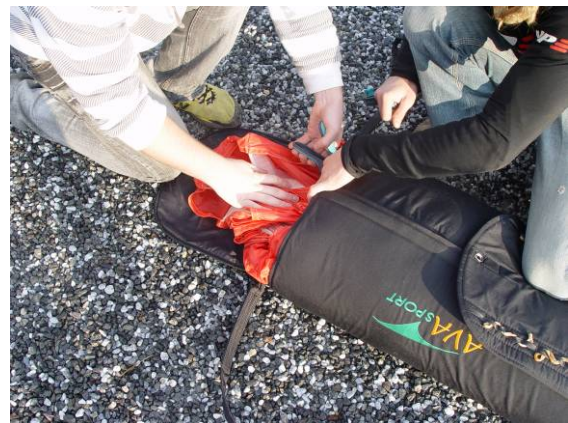
Pic. 50 remove the clamps
