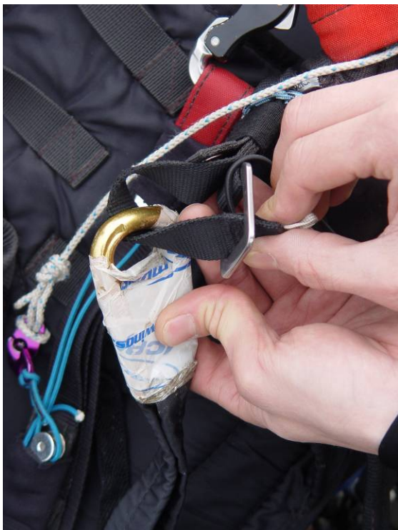
Pic. 60 the belt has to run through the karabiner and then through the release system...
