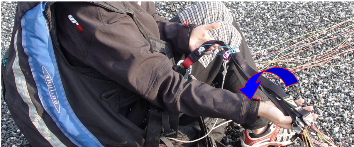
Pic. 9 at first the A-risers are facing upwards or to the outside, the right risers are turned to the right, the left ones vice versa
