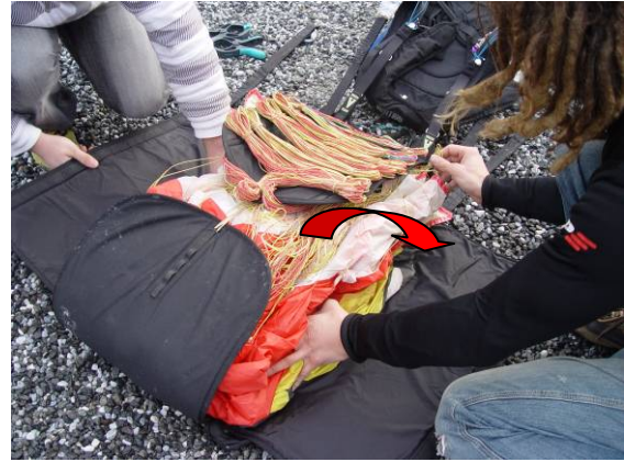
Pic. 68 turning the gliders lower side to the outside
