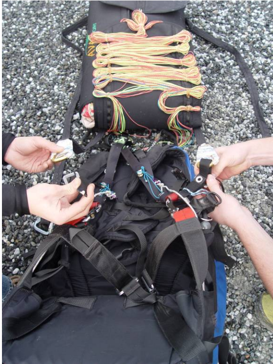
Pic. 59 attaching the release systems
