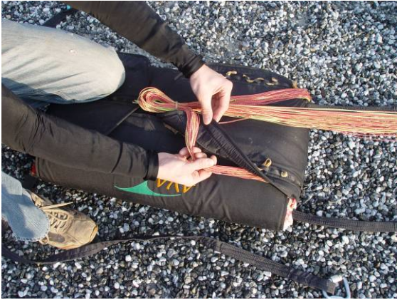
Pic. 53 put the lines under the top cover
