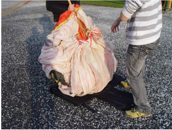
Pic. 34 put the d-bag under the glider
