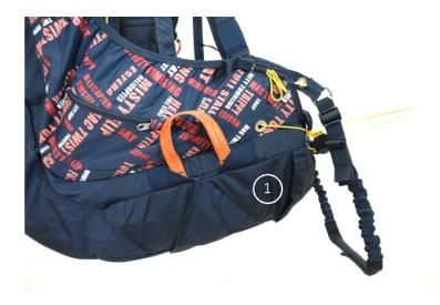
Release handle of the #1 container is placed on the left side of the harness (2) and marked as "Left handle".
