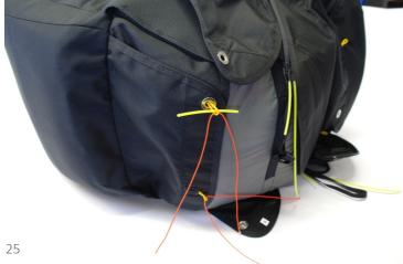
Lead the assist lines through the loops of the #6 and #6a flaps. Connect the #6 and #6a flaps and lock them with temporary pin as shown on the left.
