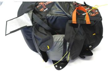
Put the rescue chute in the #2 container and close the V-strap channel with a velcro.
