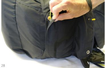
Close the pins' cover with a velcro strap and place the strap of the release handle in a tunnel on the #4 flap.
