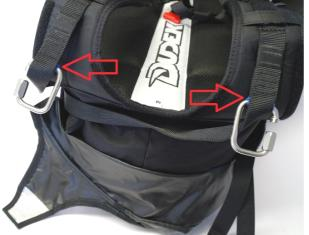
Fix the additional V-riser to the attachment points on the shoulder straps with two C6 lockable quicklinks as shown on the pictures.
