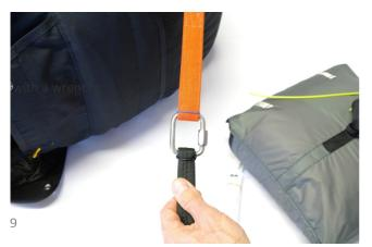
Connect the v-strap to the rescue chute riser with a lockable C6 quicklink.
