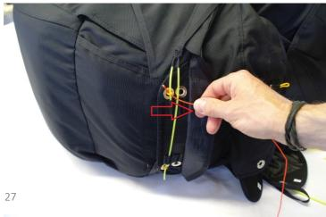
Put the tip of the longer pin into the pouch.
