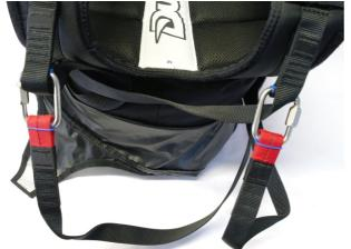
Tighten the nuts of the quicklinks with a wrench.
